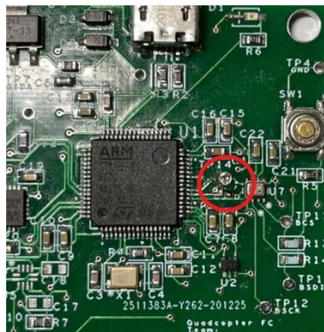
Figure 5: MISO and MOSI Switch Highlighted in Red Circle
