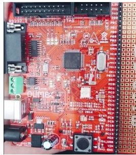
Figure 4: Image of Olimex STM32-P405 Development Board
