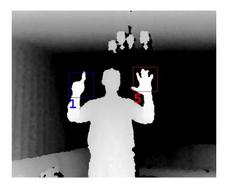
Live video feed is received from the Kinect and converted into input for the input layer. The input goes through hidden layers to distinguish identifiable traits and determine which possible alphabet sign it might be. The final layer is the output layer, where all possible outputs will reside. Upon receiving output in the output layer, a result will be sent back to the program representing the neural network's determined alphabet letter. Below shows a diagram of how the data gets processed:
