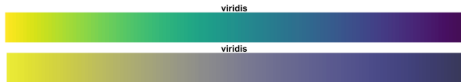
Figure 3: The Viridis color scale, and the same scale as seen by green-blind users [5].
