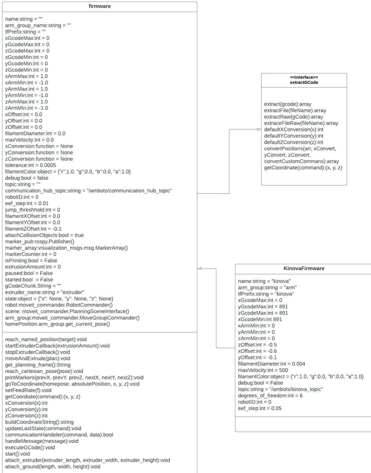
UR Firmware UML (Unified Modeling Language) Diagram:
