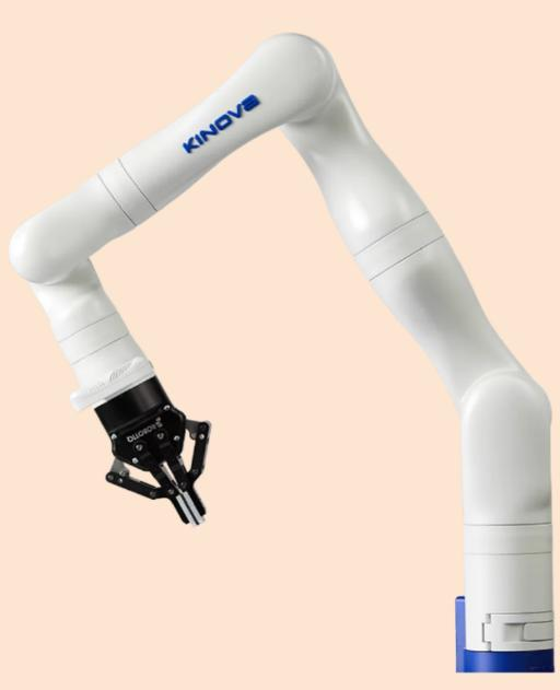
The Knova Gen3 Six Degrees of Freedom (6DOF) robotic arm is a 6-axis robotic arm. It is ROS compatible and can be simulated in both RViz and Gazebo.
