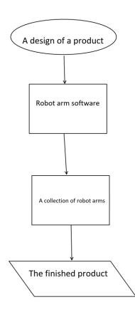
This second iteration of the design adds a software component. This software component will receive the product design and interpret it. It handles the reading of the design, the translation of the information into a language the robots can understand, and the management of the robots to produce the product. The collection of robot arms listens to the software and follow its instructions and actually perform the tasks to produce the finished product.
