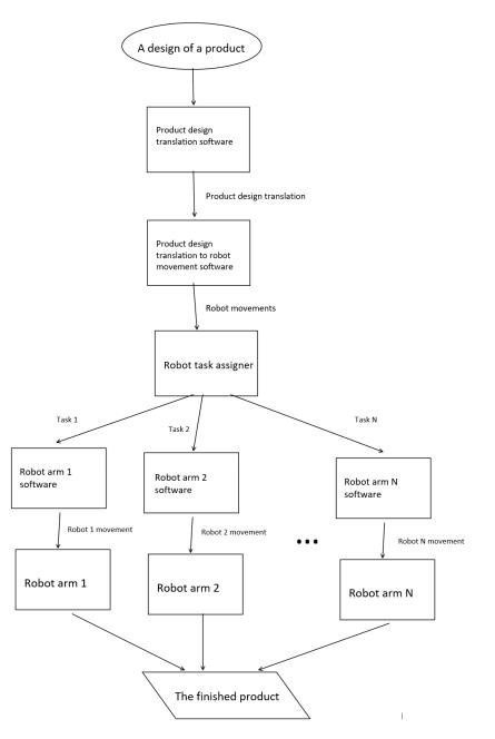
This design shows the implementation steps of the product design to robot arm movement translation. The robot arms do not understand the design of the product, so a translation layer is needed. The software will extract the necessary information from the product design. It then translates this information into movements for the robotic arms. These movements can be divided up into tasks that specific robotic arms can complete. This task assignment is done with the robot task assigner.
